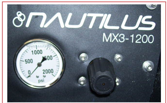
Pressure gauge & Regulator/Unloader
