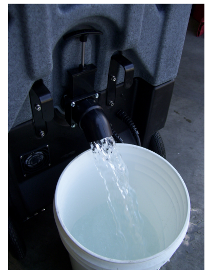
Draining the Recovery Tank
