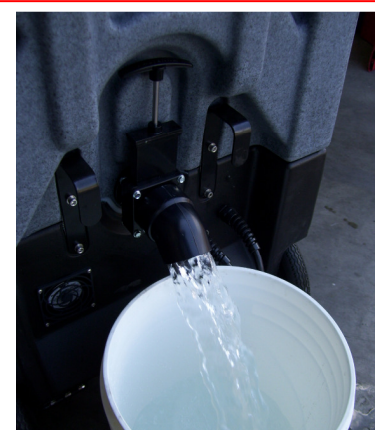
Drain water from Recovery Tank
