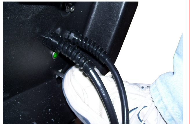
PRESSING THE PUMP PRIMING VALVE
